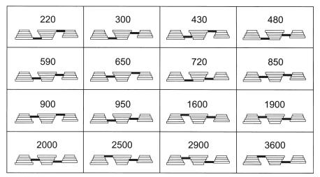
Figure C: Drill Speed Table
